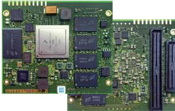
The phyFLEX-i.MX 6 SOM supports the Freescale™ i.MX 6Dual/6Quad applications processor which is ideal for use in multimedia-centric smart mobile devices, infotainment, and portable medical devices. The architecture's flexibility also allows for use in a wide variety of general embedded applications.
